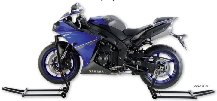
the stand does not come into contact with the fairing. If this cannot be avoided, the stand must not be used! With some steering head adaptors, a spacer is included in the scope of delivery, which creates additional distance between the stand and the fairing. You must be able to insert the steering head adaptor into the steering head tube smoothly and completely, but it must have no play, i.e. no space in which to move sideways to and fro within the steering head tube.
