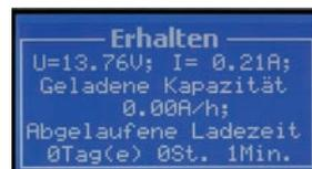
**Manual switchover to extended display** when the charger is in „Trickle charge“ (Erhaltungsladen) mode. The battery charging voltage trickle charging current, the charged capacity (residual capacity that was required to fully charge the battery), the charging time that was required.
