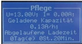
Status check by pressing the „Mode“ button or Voltage Selection button. The charger is in Maintenance mode (this is additionally indicated by the yellow „Maintenance“ (Pflege) LED). The display indicates the present battery voltage, present charging current, charged capacity in A/h, and charging time in days, hours and minutes.
