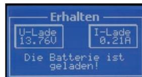
**Trickle charging:** If all the test criteria are satisfied and the battery is found to be „Healthy“ (Gut), the charger switches into Trickle mode (battery is fully charged). The display shows „Trickle“ (Erhalten) and the battery charging voltage and trickle charging current are displayed.
