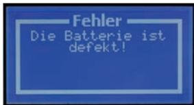
**Important!** If the battery does not pass this test, the charger considers it „faulty“, and discontinues charging. The message „The battery is defective!“ (Die Batterie ist defekt!) appears in the display.
