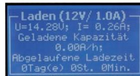
**Status check during charging** by pressing the „Mode“ button or Voltage Selection button. Present battery charging voltage, present charging current, charged capacity in Ah, and charging time in days, hours and minutes.
