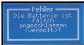
**Important!** Charger is connected to the wrong terminals. Rectify the error by changing over the battery clips. At the same time, this is indicated by the red „Wrong polarity“ (Verpolt) LED.
