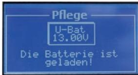
**Maintenance mode:** If the battery then remains connected to the charger, the charger will carry out the following two procedures cyclically: „Trickle“ (Erhalten) and „Maintenance“ (Pflege). These two additional programs ensure that the battery remains fully charged and in a good state after the main charging phase.
