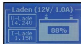
**Charging mode:** During charging, the display shows the set battery voltage, the set max. charging current, instantaneous measured battery charging voltage, instantaneous measured charging current and charge level of the battery.
