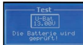
**Test mode:** If the charging current falls below a certain level while charging is in progress, charging is ended and the charger switches automatically into Test mode.
