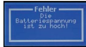
**Important!** This message appears if the charging voltage is set incorrectly, e.g. 6 V setting when a 12 V battery is connected for charging.
