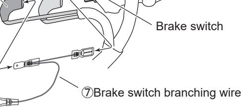
09. Connect the + wire (red) of the USB power supply body ① to the brake switch branching wire ⑦.
