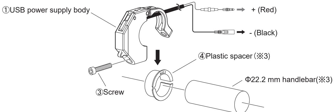
※3...On a Φ25.4 mm handlebar (or pipe), install without the plastic spacer ④.
