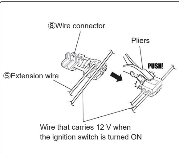
20. Connect the + wire of the USB power supply body ① to the extension wire ⑤.
