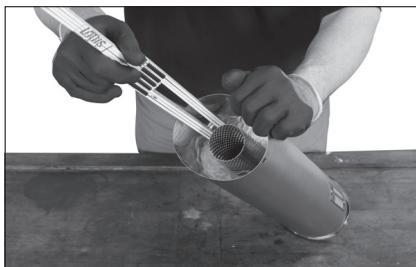
Place the end cap on the silencer so that the perforated pipe is inserted correctly into the socket and the drilled holes for the rivets align again. In the process, use the marking you have made as a guide. Align the drilled holes to each other, insert gas-tight blind rivets with the appropriate diameter into the holes, and tighten them with a riveter so that the pin on the rivet breaks off.
