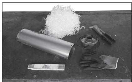
Find a suitable place where you can work cleanly and without interruptions. Lay out your tools and the conversion parts you require. Jack up the motorcycle securely. Make sure that the end cap can be removed from the silencer, e.g. by drilling out the retaining rivets. Purchase the suitable gas-tight blind rivets and a riveter for subsequent re-installation from our range.
