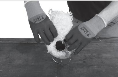
Push in more packing material with a suitable tool without pressing it too heavily. In doing so, pack the entire weighed packing material evenly up to the top in the silencer.
