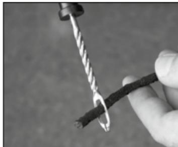
Peel a repair string from the protective film, thread it through the eye of the needle on the repair tool and apply the special adhesive.
