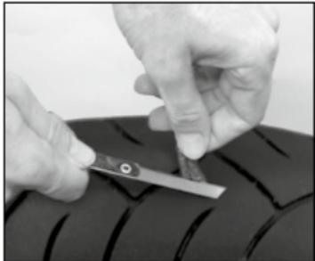
The repair string can be shortened to around 6 millimetres (measured from the outer surface of the tyre).
