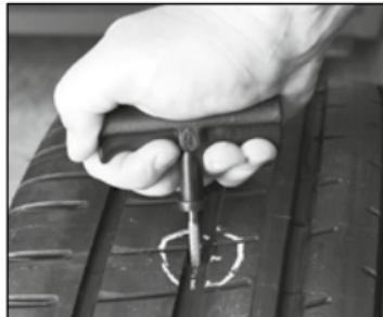
Insert the 2-in-1 repair tool (1) into the hole in the tyre. Clean the puncture by inserting and removing the awl into the course of the damaged spot multiple times. Any dirt must be removed from the puncture. The diameter of the puncture must not exceed a maximum of 4.5 mm.
