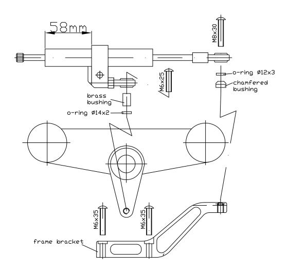
Fit the bracket on top of the gas tank fitting showing to right side. Please use the new screws M6×35mm. Install the lever under the steering head nut.
