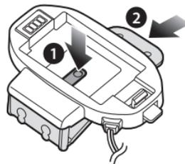
3. Align the glued surface mounting adapter and the back of the clamp kit and slide the adapter into the clamp kit until you hear a click. Make sure that the glued surface mounting adapter fits the back of the clamp kit's grooves.
