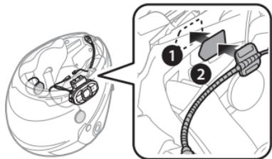
3. Align the arrows on the main unit and microphone cables and insert the microphone cable into the microphone connector.
