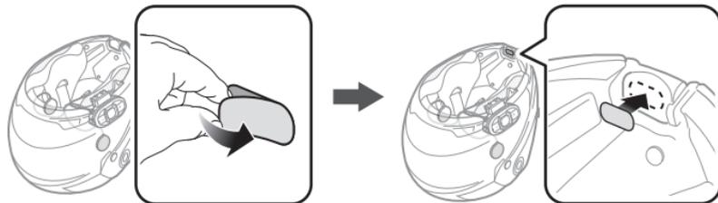
2. Attach the wired microphone to the hook and loop fastener for the wired microphone.
