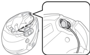
3. Align the arrows on the main unit and microphone cables and insert the microphone cable into the microphone connector.
