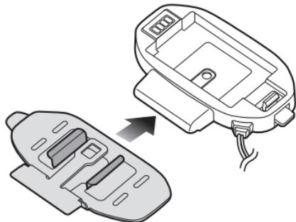
4. Push and hold the clamp kit's tab upwards. While pushing up the tab, insert the main unit into the clamp kit.
