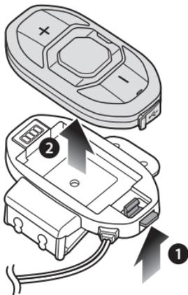
2. While pushing the latch at the center of the clamp kit, push the back plate of the clamp kit outwards to remove it.
