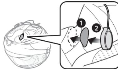
3. Connect the speaker cable to the speaker connector.
