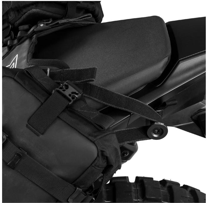
**2** Set the top straps to the longest length and loop over the alloy mounts on each side.
