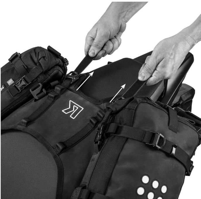
**3** Standing at the rear of the bike hold both loose strap ends and pull until the OS-BASE is firmly mounted on the seat. A strong tap downwards on each OS-PACK will help the OS-BASE slide further onto the seat.
