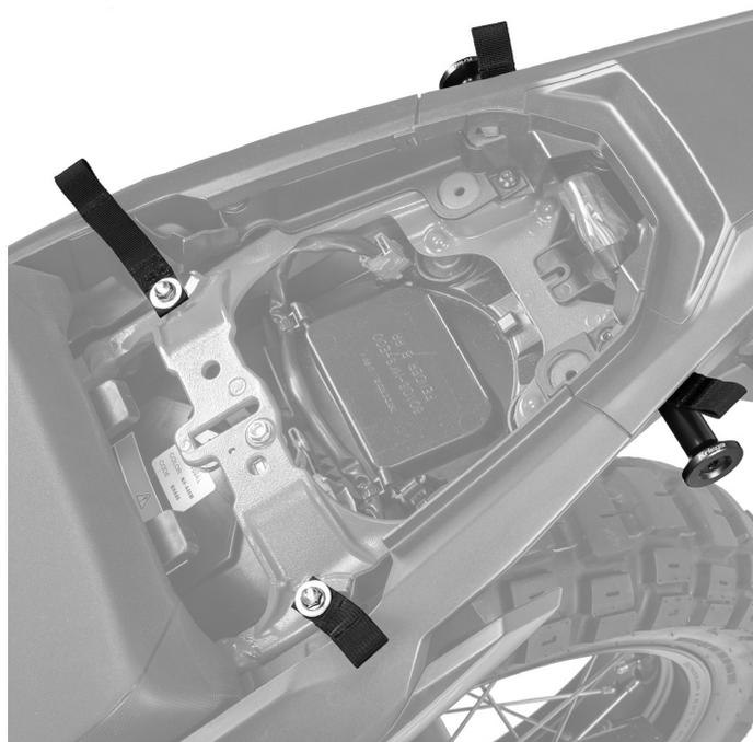
Place an M8 washer inside of the hypalon end of the two shorter bolt-on loops. Add another M8 washer and mount behind the CRF Alloy Mounts as illustrated on the front page.
