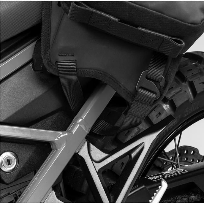
**1** Lay the OS-BASE over the motorcycle seat, forward from the final fitting position. Pass the front hook strap around the bike frame and attach the hook to the web loop so the hook is pointing down. Repeat on the other side.
