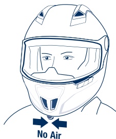
Switch to centre – ventilation disabled
