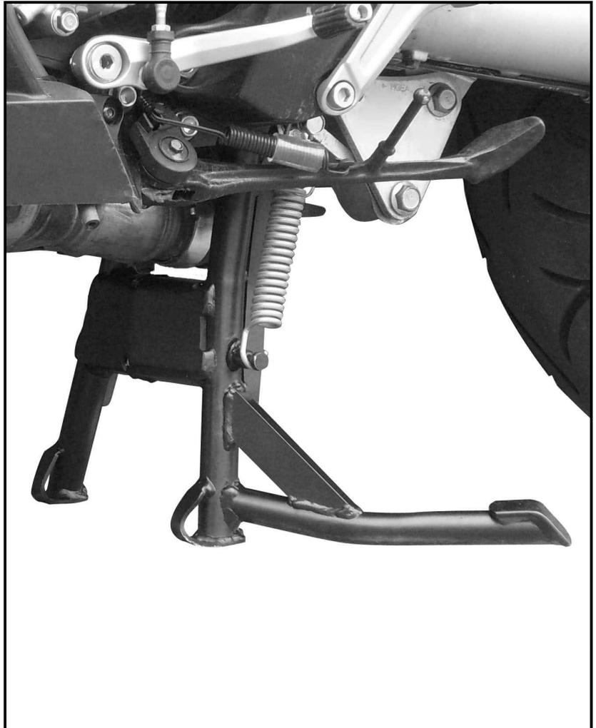
**Please check now the function of your centre stand and control all assembled screw connections for tightness!**
