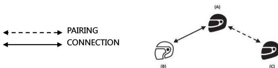
3. At this point, system C can join the intercom conference call, establishing an intercom connection with system A.
