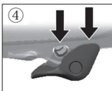
To close, push the shield down until the latch post fully engages the shield and the latch lever captures the bottom of the shield ④.
