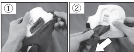
To take off the fabric covering for washing, peel the covering off over the rear edge of the cheekpad assembly until all the fabric is on the face side surface. Then draw the covering through the opening by grasping the rectangular collar and pulling.
