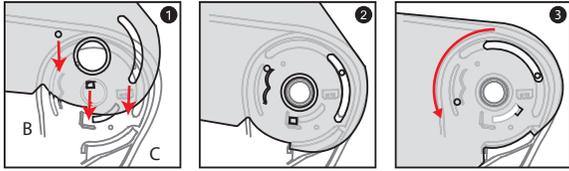
1. Align and insert the top of the shield guide into the plate-gear guide.
