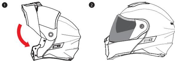
Pull the chin bar downward to completely cover your face and chin. Listen for "click" sound to ensure that the chin bar has locked into its full closed position.
