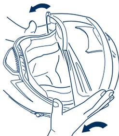
3. Make sure that the visor mechanism is functioning properly by opening the visor once to its maximum extent.
