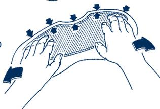
4. Check right around the visor to make sure that the silicone seal fits tightly and uniformly against the outer shield. It is only if it does that the visor can be guaranteed to prevent misting.
