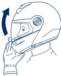
2. The Bowden cable mechanism will then release both locks and you can pivot the chin section up to its uppermost locking position.
