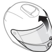
2. Loosen the two short screws on the cover of the helmet with the included allen wrench, and then remove the cover.
