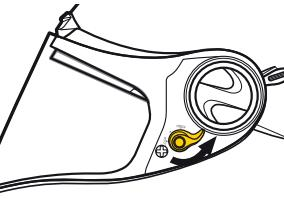
To lock the faceshield, turn locking-lever counter clockwise to the 2 o'clock position approximately.
