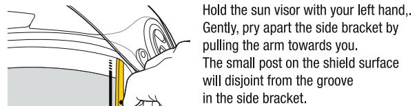
Release the shield from the clasp, pulling downwards slightly. With one side now disjointed, pry apart the other side to completely detach the sun visor.
