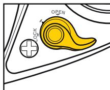
NOTE : When the lever is positioned at 4 o'clock, the shield is closed, but it is also unlocked.
