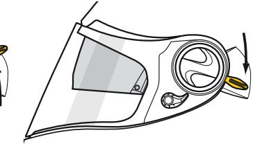
To lower the sun visor, simply pull the sun visor retraction lever down.
