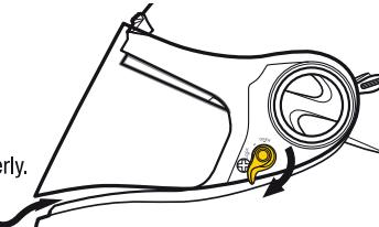
To unlock the faceshield, turn locking-lever clockwise to the 7 o'clock position until it unlocks. Test faceshield now to check if it's unlocked properly.
