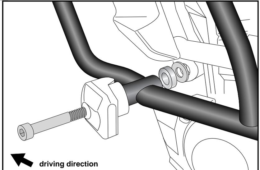
**When mounting with skid plate the original washer and the alu spacer will not be used.**
