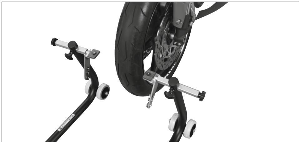
When inserting the front wheel supports and V-adapters, make sure that they are aligned correctly—see assembly examples.
