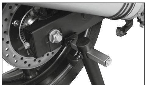
Adjust the angled universal adapters on the Rothewald Paddock Stand to the width of the rear-wheel swing arm. To do this, a second person must hold the vehicle firmly to keep it upright. Bring the supports up to the motorcycle's swing arms from the rear, and adjust the adapters so that they fit fully under both swing arms. The full width of the swing arms must rest on the supports so that the motorcycle is held securely.
