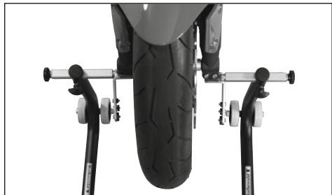
Make sure the adapters are a good fit in the opening and do not have too much play. Lock the supports with the tommy screws.
