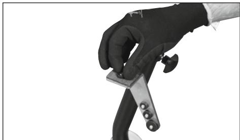
First check that the fork tubes are open at the ends, and measure the size of the opening. There are four different sizes of adapter in total: 12 mm, 14 mm, 16 mm, 22 mm. Select a suitable size and screw the adapter onto the thread of the felt protector. To do this, you may need to remove the adapter from the paddock stand beforehand.
