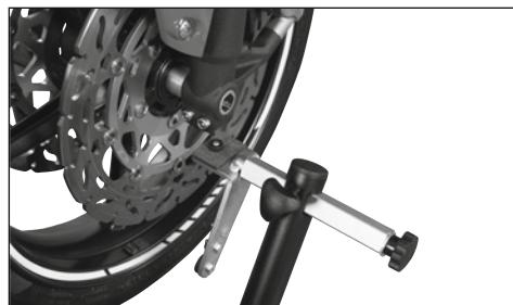
The Rothewald Paddock Stand supports for open fork tubes must be adjusted to the width of the front fork. To do this, a second person should hold the handlebar straight. Position the supports with the correct adapters under your motorcycle's fork tubes from the front. Adjust the supports so that they fit fully under the two fork tubes, and fit the adapters into the opening/hole in the fork tubes.
