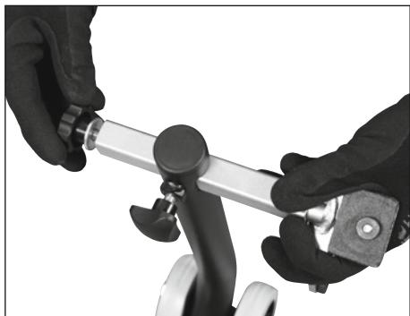
The two Rothewald Rear Paddock Stand models are suitable for an inner swing-arm spacing of 270 mm to 360 mm.
