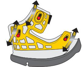
For installation, reverse the above process and double check that the cheek pad snaps are in the down location. They may have slid up upon removal (as part of the Emergency Release System).
