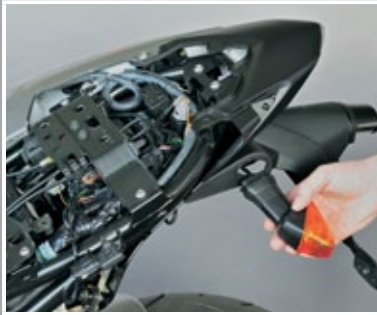
Take off tail fairing and remove turn signals
