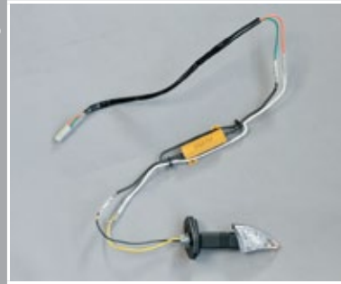
Correctly wired: turn signal, resistor, adapter cable
