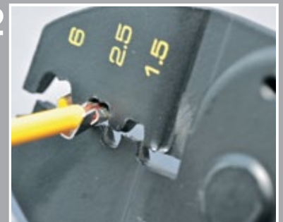
Multifunctional crimping tool for Japanese connectors without coloured markings
