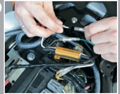
Resistor connection at the rear
