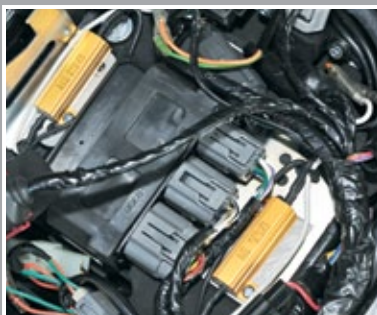
Resistors fitted underneath the seat
