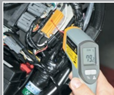
Infrared thermometer reads 79°C after a few minutes
