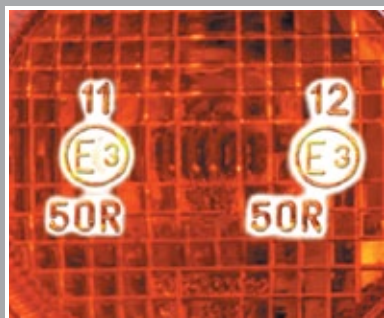
Important: Only use turn signals with an "E" mark
